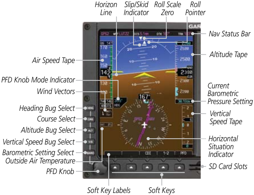
Figure 2-1 PFD Description (Ground Pointer Mode)
